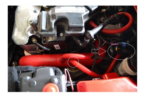
Make sure the intercooler side of the pipe is fully on. They will go over the lip on the opening. (Use soap and water for lubrication!)
