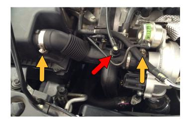
• Unclip the electrical connector ( ) from the factory diverter valve, then remove the 3 bolts ( ) that hold it to the turbo.
