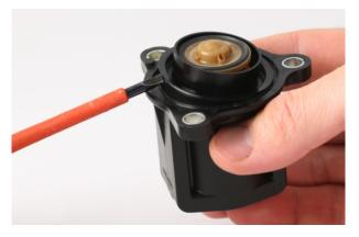
Assemble the GFB parts onto the factory solenoid body as shown in the exploded view below, making sure to use the GFB-supplied plunger spring, and the yellow o-ring removed from the factory valve. Apply some engine oil to the piston during this process.
