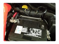
I. Disconnect battery both positive and negative terminals.
