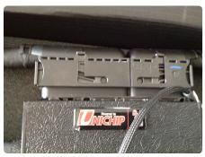
5. Next, you have to remove the Unichip plugs from the harness. This can be tricky as there are no yellow locking clips and no levers to lift to unlock plug slides and plugs are tight.
