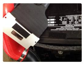
20. You can mount the booted Unichip on the battery by securing it with the supplied velcro. Or the Unichip can be velcroed to the back of the ECU (near the brake fluid reservoir).
