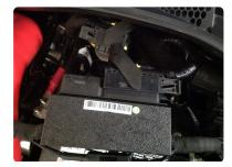
II. Insert stock ECU harness plug on Unichip harness, \*\*making sure harness sits snugly and nicely\*\* level before lowering arm to lock slide. Relock yellow clip.
