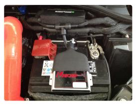
21. Finished look. Make sure to do a hard reset by disconnecting both battery terminals. Follow Unichip break-in procedure found on Eurocompulsion website and enjoy!
