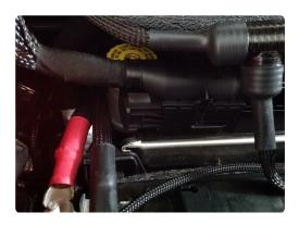
13. Take one Unichip harness plug and insert into stock ECU plug, again being very careful to seat plug level and snugly before pushing in locking slide to secure plug. To seat Unichip harness plug well, you may need to move the positive battery cable out of the way for the left smaller plug as well as the fuse box harness out of the way for the larger plug on the right side.
