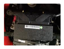
12. Repeat process to insert other stock harness plug into Unichip harness, again making sure plug sits snugly, level and securely before lowering lock arm. Relock yellow clip.
