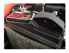
17. Take you Unichip and observe the orientation of the plug inside the rubber boot to make sure you plug it in correctly.
