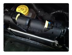
2. Disconnect stock ECU plugs from stock harness. Slide yellow locking clip first. Then, lift locking lever up all the way to disengage locking plug slide. (You will NOT be able to unplug both stock plugs at the same time, only one at a time)
