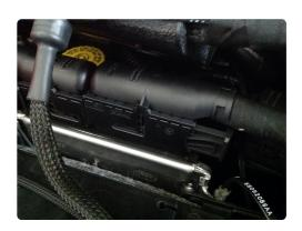
14. Repeat process to insert remaining Unichip harness plug into stock ECU. Push locking slide back in.
